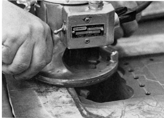
Figure 15: Damage Removal with Hand Held Router.
